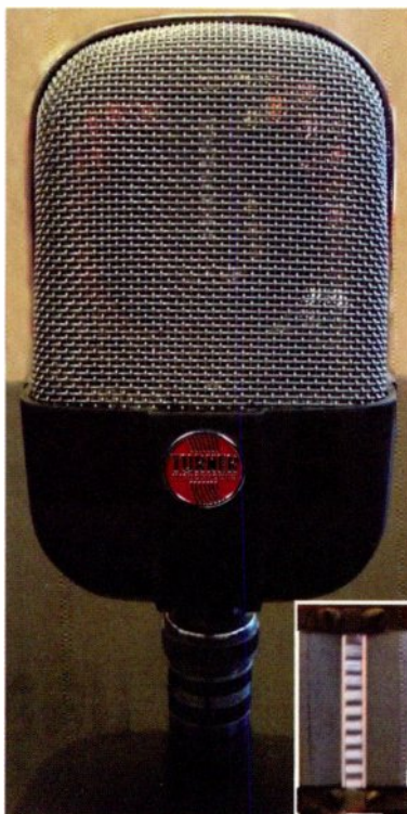
Fig. 1: The Turner Model 87 ribbon microphone. The inset shows the ribbon John Rausch corrugated and installed.
