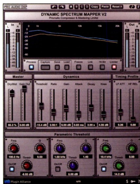
Figure 1: The Pro Audio DSP Dynamic Spectrum Mapper V2 uses FFT-based multiband compression to make your mix's tonal balance dynamically approximate or match that of a captured spectrum.
