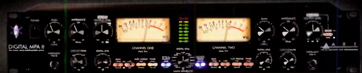
DIGITAL MPA II Two Channel Class-A Tube Mic Preamp with Flexible AES/EBU, S/PdIF and ADAT Digital I/O TWO CHANNEL TUBE MIC AMPLIFIER with DIGITAL OUTPUTS
