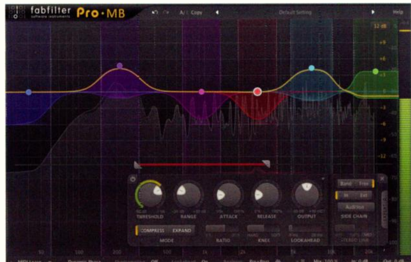
Fig. 1: Pro-MB offers six independent bands for implementing upward and downward compression and expansion. Each band has its own sidechain with tunable bandpass filter (shown here as a red horizontal line above the GUI's control knobs).
