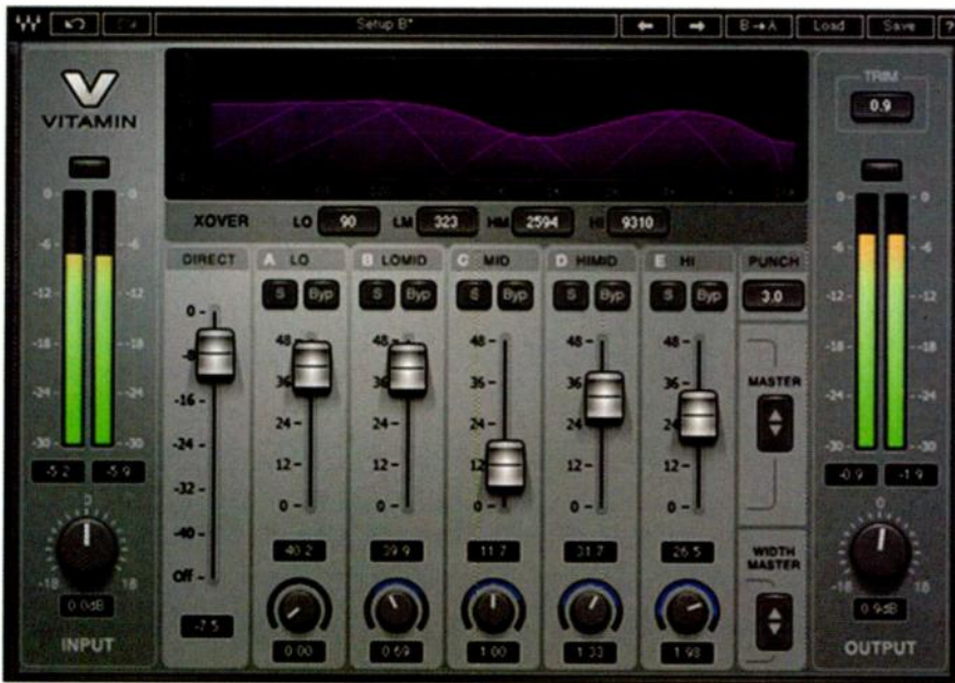
Waves Vitamin Sonic Enhancer uses multiband processing to add harmonics, adjust stereo imaging and brighten transients. Example settings for use on stereo acoustic guitar are shown here.
