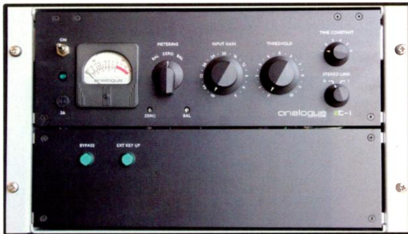
The AT-1 uses 12 tubes: 6386LG, 6084, 5651, 12AX7, 12BH7, 6BL7, 6L6GTA, and GZ34.
