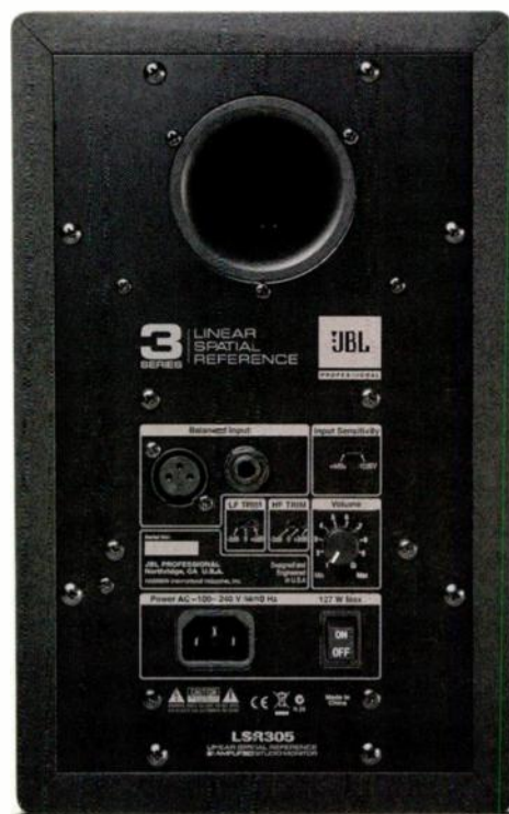
Fig. 2: Balanced inputs, two filters, a detented volume control and an input-sensitivity switch grace the LSR305's rear panel.
