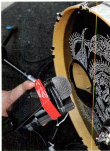
The drum kit is entirely Neumann KM 184s, though the kick drum has a Shure Beta 52 inserted.
