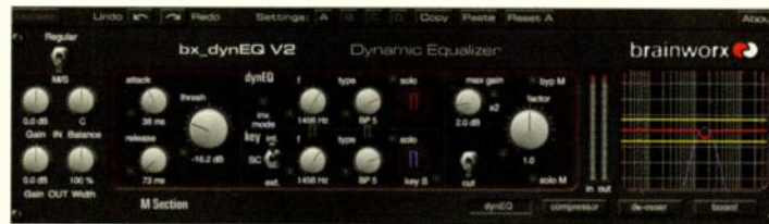
Fig. 3: Brainworx bx_dynEQ takes the edge off lead vocals during choruses. The section of the GUI for the side channel (which is bypassed) here for clarity's sake.
