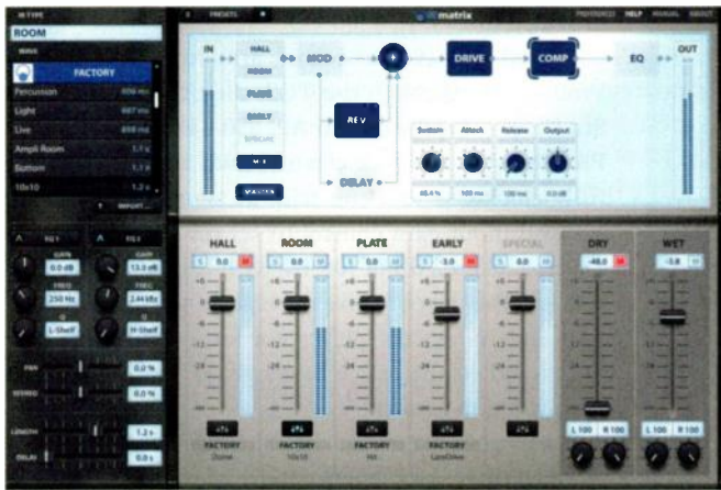
Figure 1: REmatrix can mix five convolution reverbs with five other effects and EQ. The Master effects iGUI top-center) and a room IR's Extended Controls panel (left side) are shown here.
