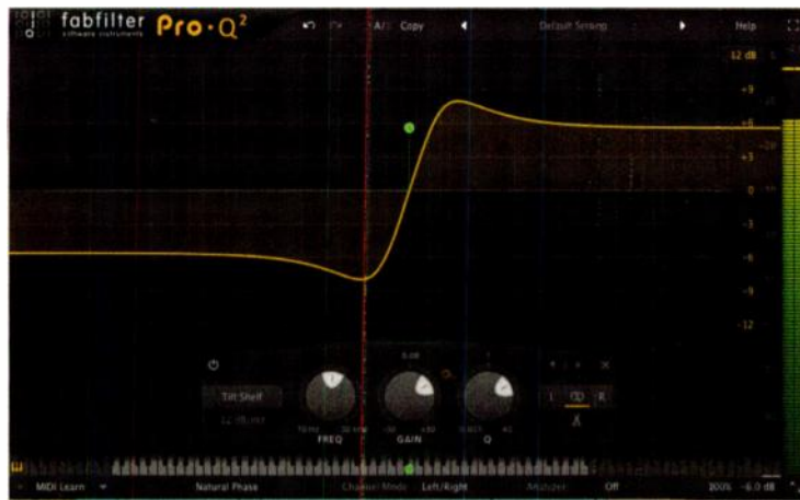
Figure 2: A high-Q setting for a tilt-shelf filter creates classic overshoot response. The plug-in's Piano Display mode replaces frequency titling with a virtual keyboard along the x-axis.
