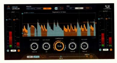
Drum Leveler features high- and low-threshold settings, plus a sidechain switchable between bandpass and band-reject modes.
