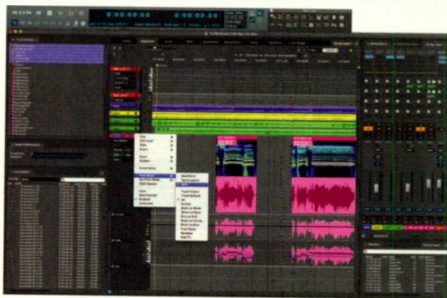
Fig. 1: As seen here in the bottom half of the center of this view, DP 9 can display audio tracks as a waveform and in a spectrogram at once. Separate lanes show automation data directly below each audio track.
