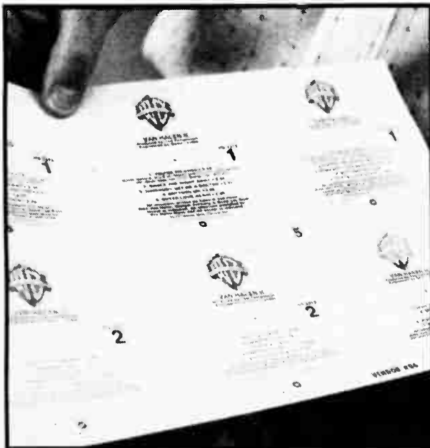
Record company label "backdrop", which will be applied during pressing.
