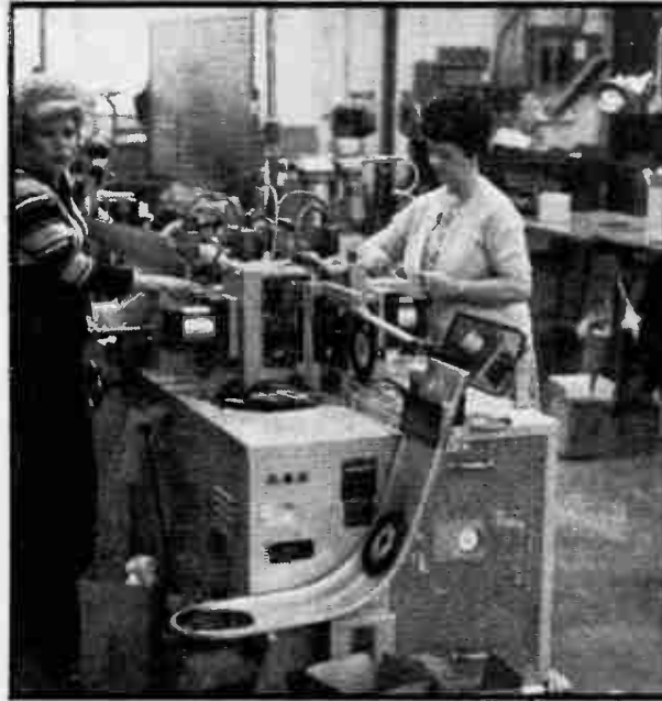
Finishing station for 7-inch singles where labels are applied and records boxed.
