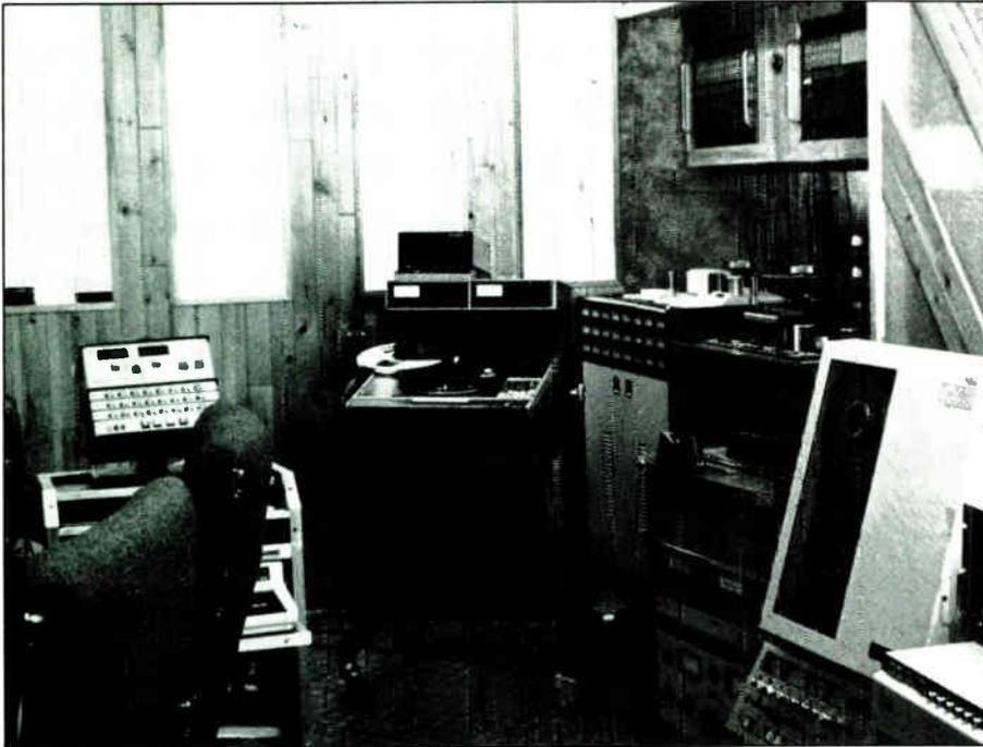
*"The Backroom" at Universal—a complete video sweetening facility housing two 24 track recorders, a unique Ampex 1200 that can be fitted with different headstacks, the house synch-generator, and all necessary synchronization gear.*
