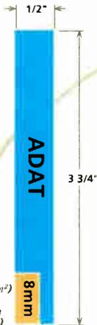
Actual microscopic comparison of the ADAT tape format and the 8 track, 8mm helical scan format (enlarged approximately 100 times).
