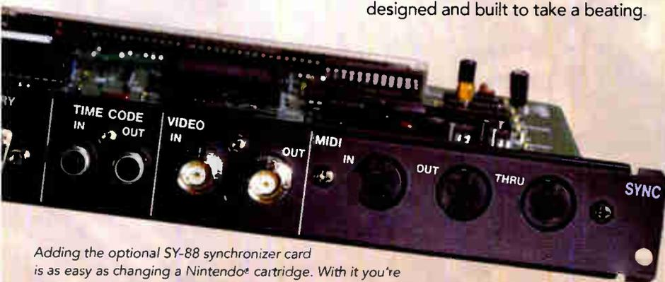
Adding the optional SY-88 synchronizer card is as easy as changing a Nintendo® cartridge. With it you're SMPTE and MIDI compatible. And no matter how many DA-88s you have locked up, you need only one sync card. Other optional accessories include AES/EBU and SDIF2 digital interfaces allowing the digital audio signal to be converted for direct-digital interfacing with digital consoles, signal processors and recording equipment.
