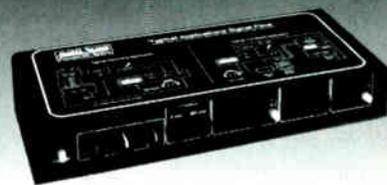
3 Inputs HARD-WIRED to three thru outputs allow custom monitor mixes from a single send. UNIQUE ability to PASS THRU UNCHANGED signals—powerful amplifier drives ALL types of headphones.
