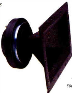
outstanding pattern control (90° X 50°) and exhibits the lowest midband distortion we have ever achieved in large format systems. Equally important, the 2447J compression driver extends high frequency response well above 18 kHz, virtually eliminating the need for a separate tweeter.
