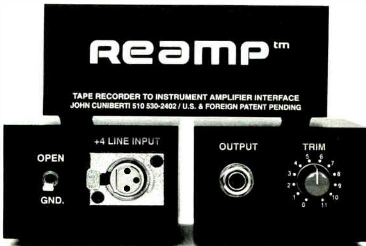
REAMP is about the size and shape of the popular Countryman direct box. Because it is passive, there are no batteries to change, and it is RF-protected. On the input side is a ground lift switch and a female XLR +4dBu connector in which to plug your tape track output. On the output side is a volume trim pot (yes, it goes up to 11) and a 1/4-inch jack for connection to an amp.
