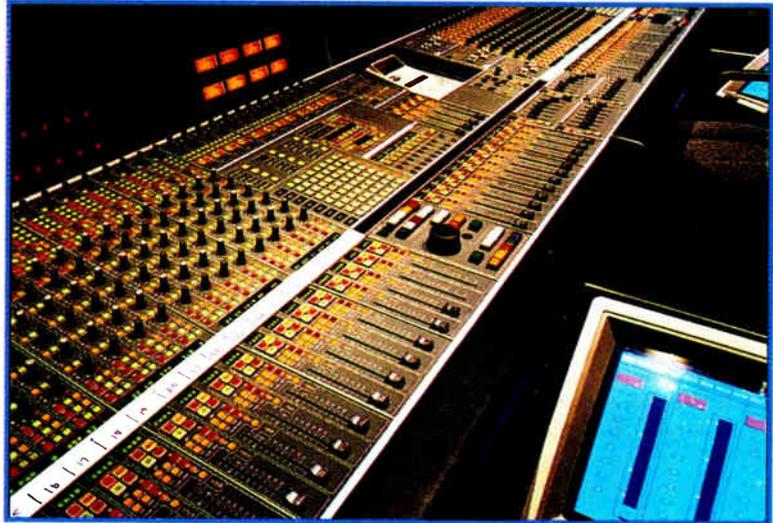
to any experienced mixer or re-recording engineer. Software-controllable functions are handled via a high-res, touch-sensitive VDU at each of the music, effects and dialog mixing stations (assuming a conventional three-person console layout). Multiple pages on the MPC's Interactive Touchscreen Interface (ITI) are quickly accessed from the menu bar located at the top of the display.
