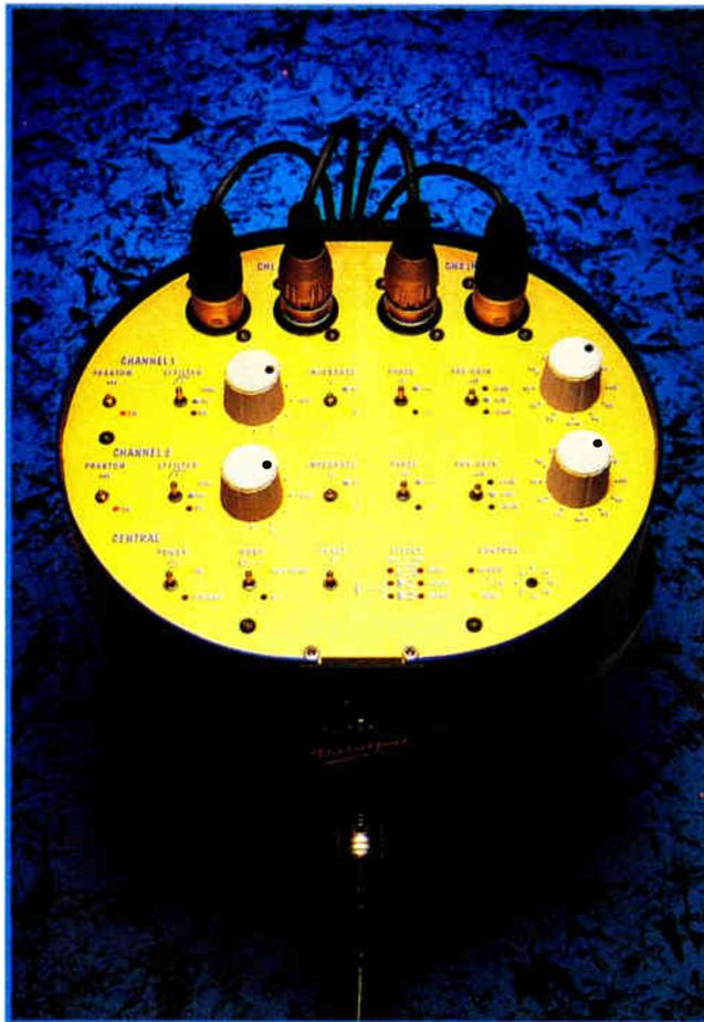
switch (that's located on the unit's underside) at all: It changes from "on" to a Standby mode, where power to the relays and phantom circuits is disconnected. The Paintpot offers a feature rarely found on preamps; each channel has a high/low impedance switch for matching the preamp loading to the
