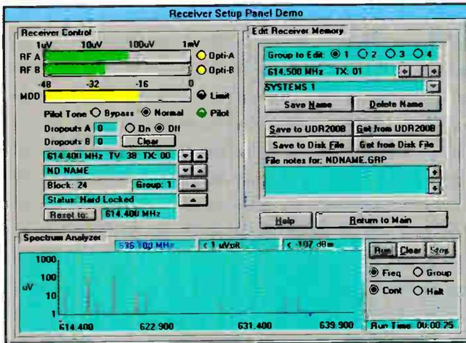
The UDR200B receiver is supplied with LecNet™ software to run under the Windows® operating system. The control panel for an individual receiver shown here includes indicators of present receiver settings and levels, an edit section to make changes, store and retrieve files, and a spectrum analyzer section that provides a spectral plot of the tuning range of the receiver.
