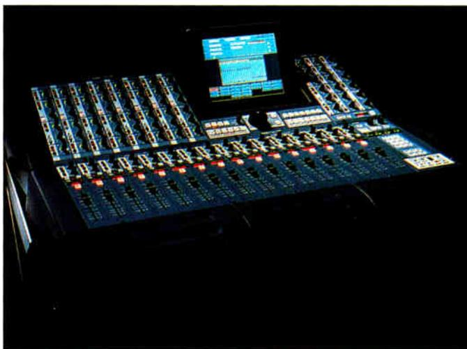
issue MMC data. Metering is via onscreen meters (users can select preferred meter type, ballistics, scaling, etc.) and/or an optional meter bridge with VU, plasma or digital meters. Onscreen phase metering is standard.
