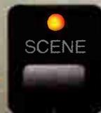
Every mixer setting, including virtual tracks and effects, can be saved as a scene. Store a snapshot of a mix when you're bouncing tracks. When you need to re-bounce the tracks to adjust some of the levels, you still have the originals saved on virtual tracks.
