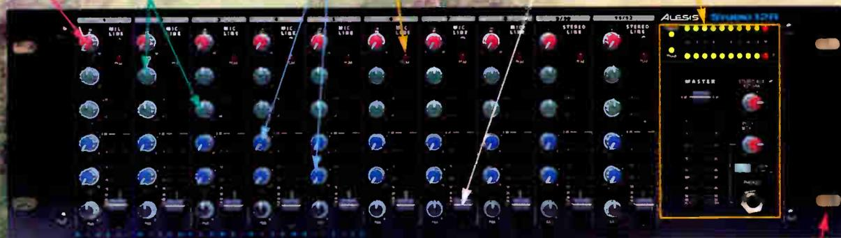
48V phantom power for use with high-quality condenser microphones.
