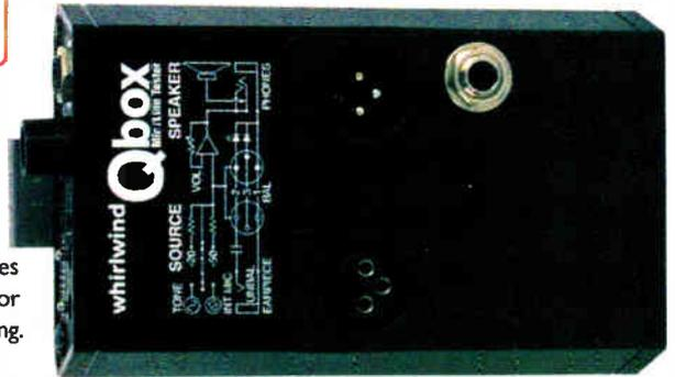
The PHASE REVERSE is the quick cure for an "out of phase" mic
