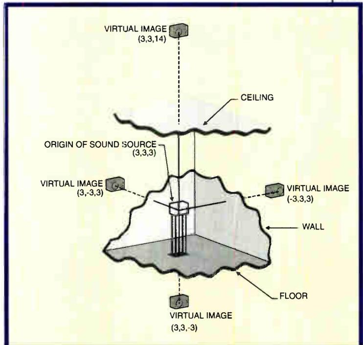
Figure 2: Speaker-Boundary Interference is caused by the combination of sound from real and "virtual" (boundary reflection) speakers.
