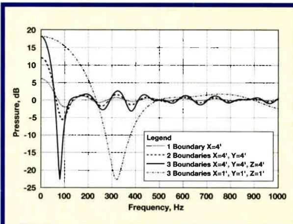
Figure 3: Speaker-Boundary Interference Response for several loudspeaker positions in a corner
