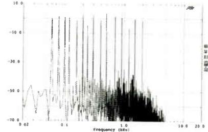
**Figure 4: Spectral contamination test compares a series of input signals (tall spikes) to speaker output. Clarity is average, with self-noise 40 dB below input signals.**
