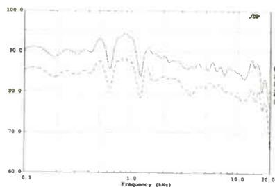
**Figure 1: On-axis and 30° off-axis frequency response. Very flat on-axis response and fairly smooth off-axis response.**
