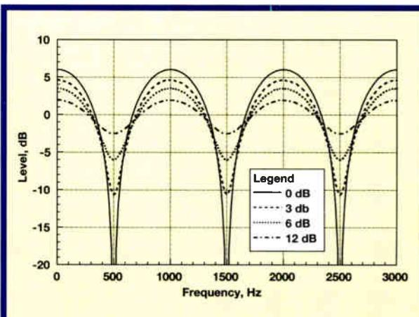
Figure 4: Comb filtering with one reflection delayed by 1 ms with attenuation of 0, 3, 6 and 12 dB relative to the direct sound
