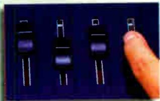
*Just push the Wedge's edit button and start adjusting your reverb with the four edit sliders. It's easy to get creative with the Wedge's powerful parameters like decay, frequency damping, swirl, early reflection room shape, width, density and diffusion.*
