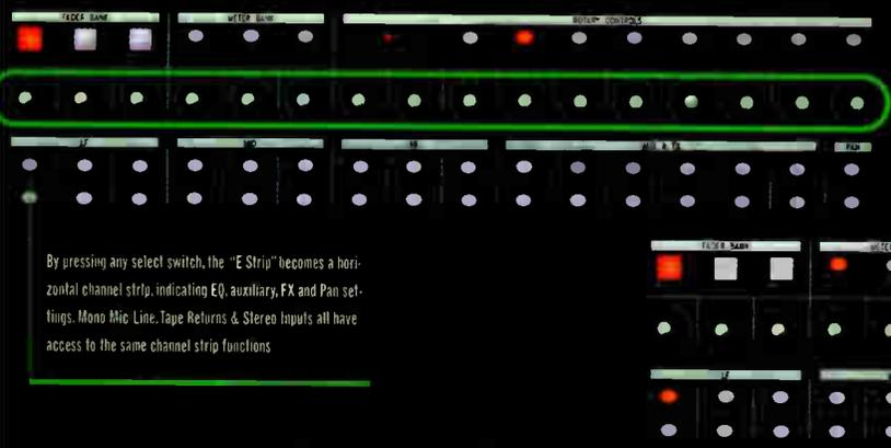
By pressing any select switch, the "E Strip" becomes a horizontal channel strip, indicating EQ, auxiliary, FX and Pan settings. Mono Mic Line, Tape Returns & Stereo Inputs all have access to the same channel strip functions
