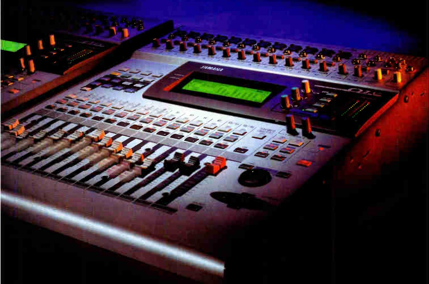
Our new 01v digital mixer has everything you need for top quality recording and live sound. You get 24 inputs, 6 busses, 6 aux sends, direct outs, 12 mic preamps with phantom power, 34 parametric equalizers, 22 limiter/compressor/gates, two 32-bit effects processors, motorized faders, snapshot memory
