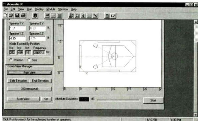
Figure 1: Based on the 8x10x18-foot room dimensions, Acoustic-X predicted this optimal speaker positioning.
