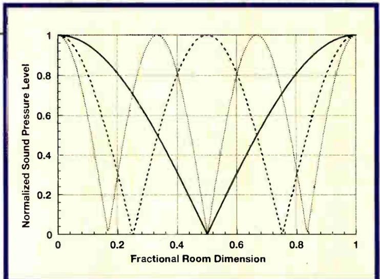
Figure 1: Normalized energy distribution of the first three modes in a room: The solid line is the fundamental, the broken line is the first harmonic and the dotted line is the second harmonic.
