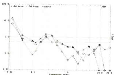
**Figure 3: Distortion (THD+N =  $\Delta$  trace; 2nd Harmonic =  $\circ$  trace; 3rd Harmonic =  $\square$  trace) remains under 1% from 100 Hz upward.**
