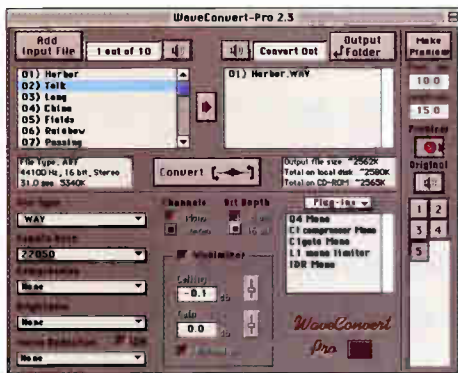
Figure 3: WaveConvert Pro's main window is used to create input and output file lists and to define processing parameters, including multiple Waves plug-ins. Up to 16 previews may be created and compared using the preview section on the right.
