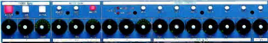
...A HORIZONTAL INPUT CHANNEL WITH FULL EQ, AUX AND PAN FACILITIES...
