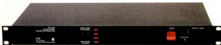
filtration and four stages of power up/down via eight rear panel AC outlets. Capacity is 15 amps (1,800 watts). Four preset intervals ensure that equipment is powered up or down at intervals of 1, 5, 10 and 30 seconds. Manual settings offer intervals of up to 240 seconds. The front panel features a "go/no go" LED display and a single "always on" AC outlet. There are two additional "always on" AC outlets on the rear panel. Price is \$390.
