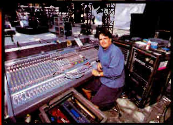
"The only open mic I have in the monitor rig is Shirley's vocal mic," says Brian Kaeffke. "I only use the overhead on two songs; the rest are direct inputs. I'm using the Midos XL-3 console; I think it has one of the best sounding preamp EQ sections made."
