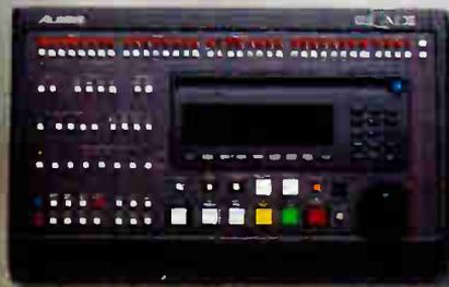
An all new remote/autolocator, the CAD<sup>1</sup>, provides control of up to eight M20s from hundreds of yards away. Remote metering in the control room is made possible by the new RMD<sup>2</sup> meter display.
