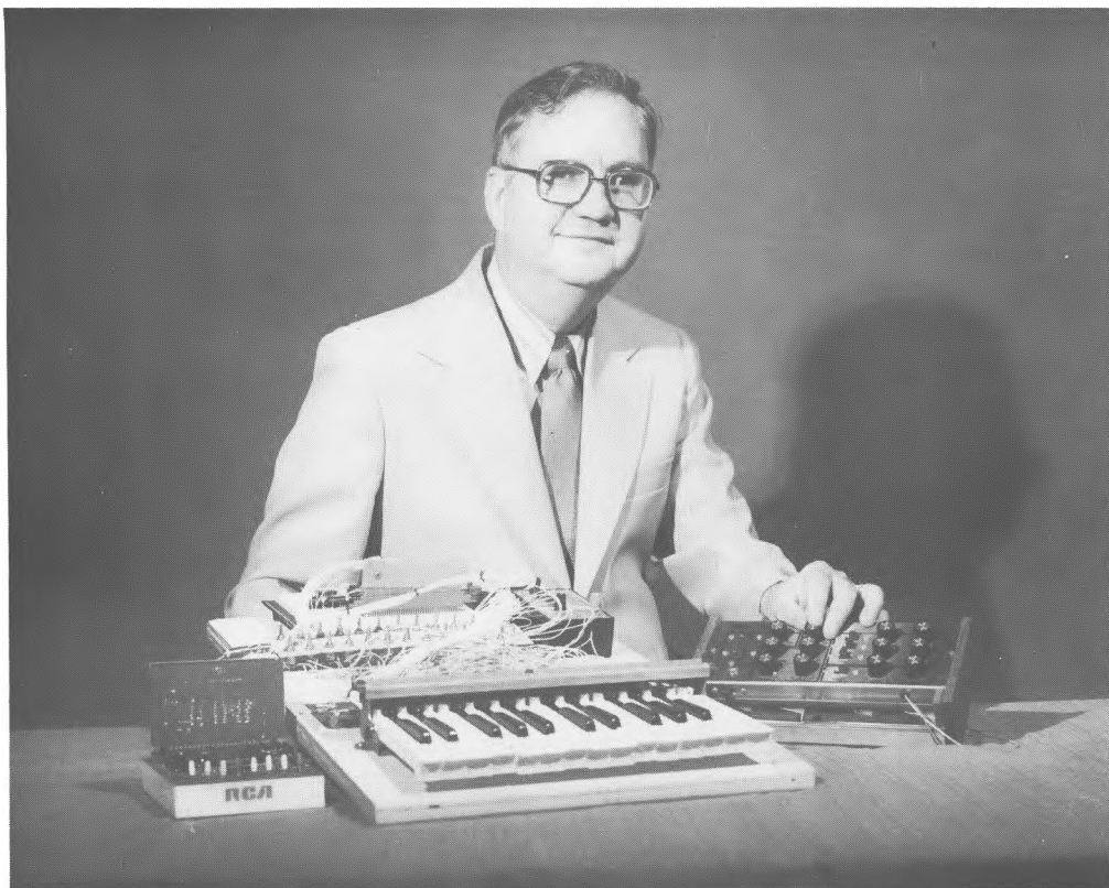
Author with his Combo. At left is the RCA COSMAC Microtutor; at center (front to rear) are the keyboard, interface, and attenuator; synthesizer at far right.
