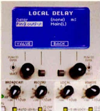
**Synchronic™** measures the audio delay between the main and fill speakers, then automatically sets the time delay necessary to make the audio synchronous—eliminating delay and phasing problems
