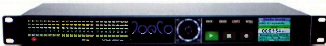
BlackBox records audio as Broadcast Wave files to USB2 disk drives, USB thumb drives, or SDHC card via USB2.
