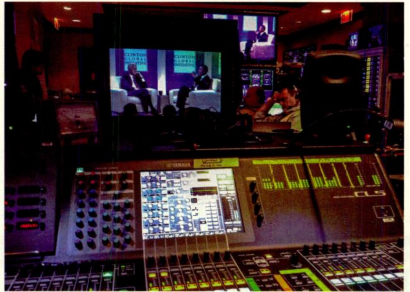
A string of Yamaha CL series consoles and a Dante network handle audio routing and distribution requirements for the annual Clinton Global Initiative.
