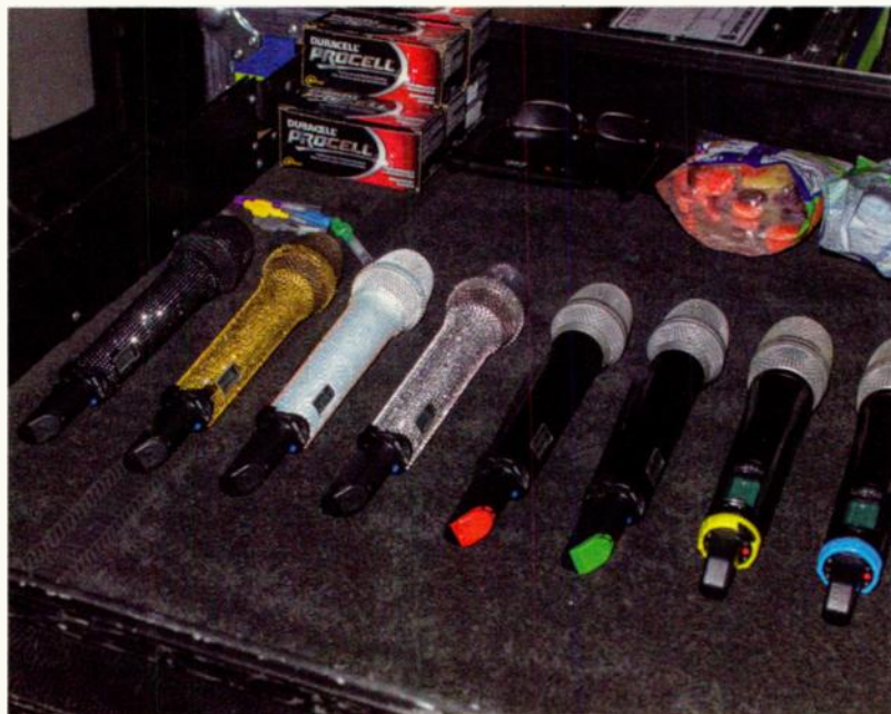
The tour carries a selection of Sennheiser 5200 series wireless handhelds with 5235 heads. Guess which ones are Cher's.
