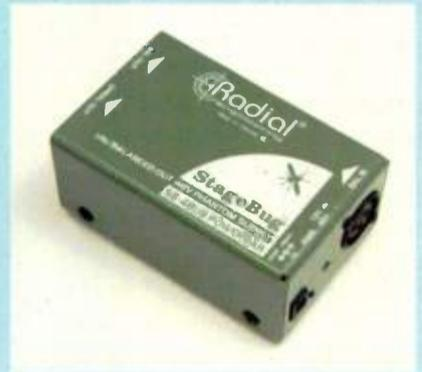
The design begins with a solid steel outer shell with XLR female input to connect the mic. Power is derived from a 15VDC supply and an internal non-radiating charge pump elevates the voltage to 48V for standard phantom power use or it may be set to 12VDC. A choice of balanced XLR or unbalanced 1/4" output is available.
