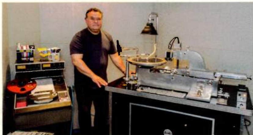
Mastering Engineer Ron Leeper in between Sound Affair's Ampex ATR-102 reel deck and Scully lathe.
