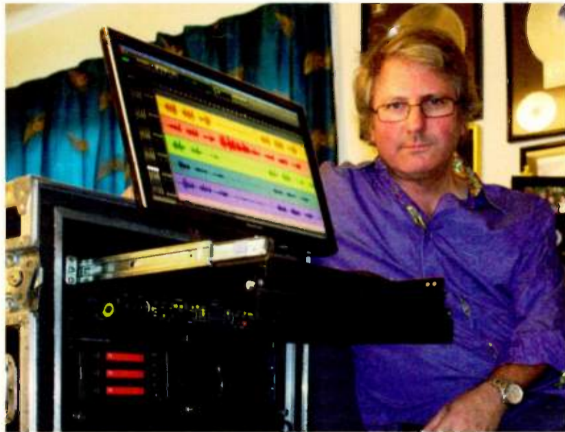
Brad Madix of Diablo Digital with one of the company's live multitracking solutions, featuring Avid Pro Tools|HD software running on a Mac Mini in a Sonnet housing that also provides storage and console interface.
