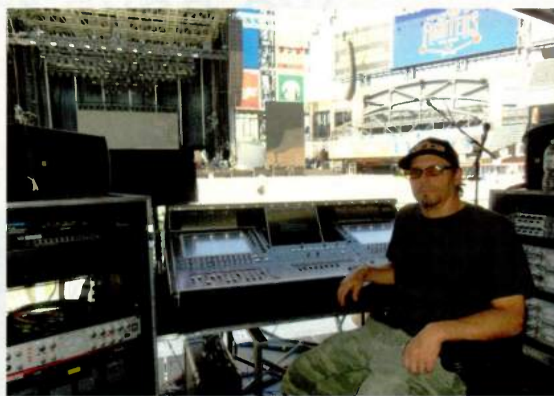
FOH engineer Bryan Worthen treats his DiGiCo SD5 console like an analog desk, eschewing snapshots and so forth, as he sends his mix to the massive L-Acoustics K1/K2 PA, seen here in New York's CitiField Stadium.
