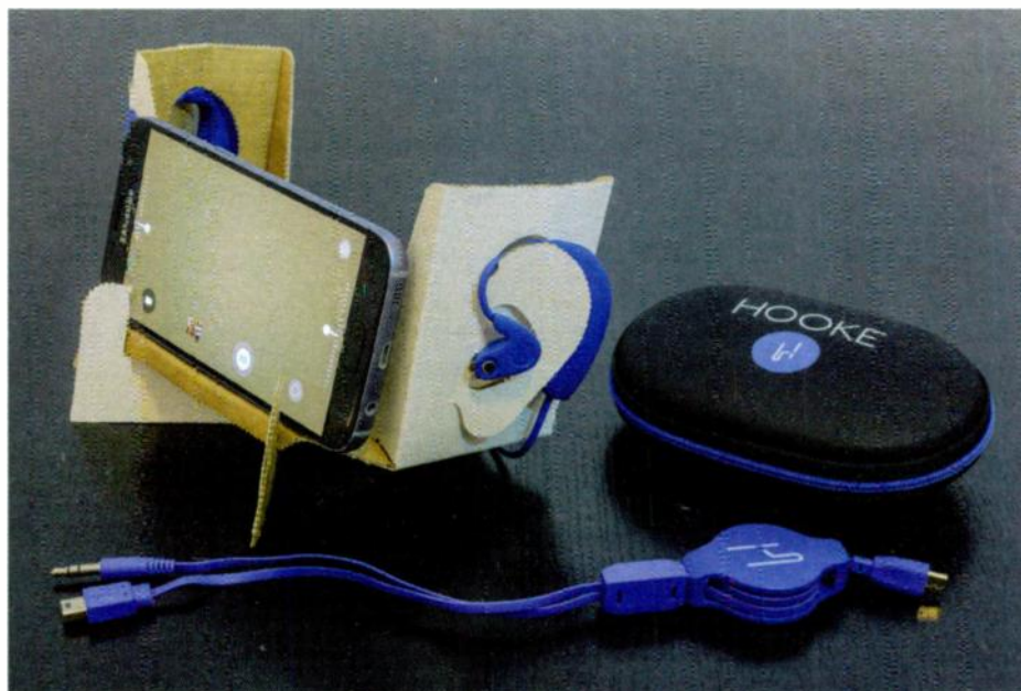
Verse, a pair of Bluetooth headphones with integrated binaural microphones, is well thought out, to the point where its box is pre-cut so that users can use it as a dummy head to hold both earpiece/microphones and a smartphone.
