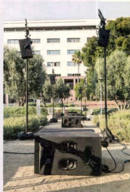
Delay 2 between Zone 2 and 3: flown Y10s plus J-Subs
