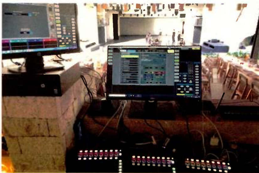
The venue’s control center consists of three IP8 remote controllers and a touch-enabled computer running dLive Director.
