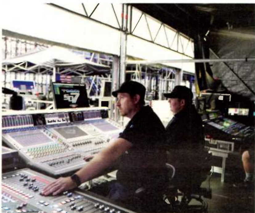
(L-R) Artist monitor engineer James Berry, FOH engineer Stephen Curtin, and band monitor engineer Jimmy Corbin at the On the Run II tour's primary DiGiCo SD7 FOH mixing console
