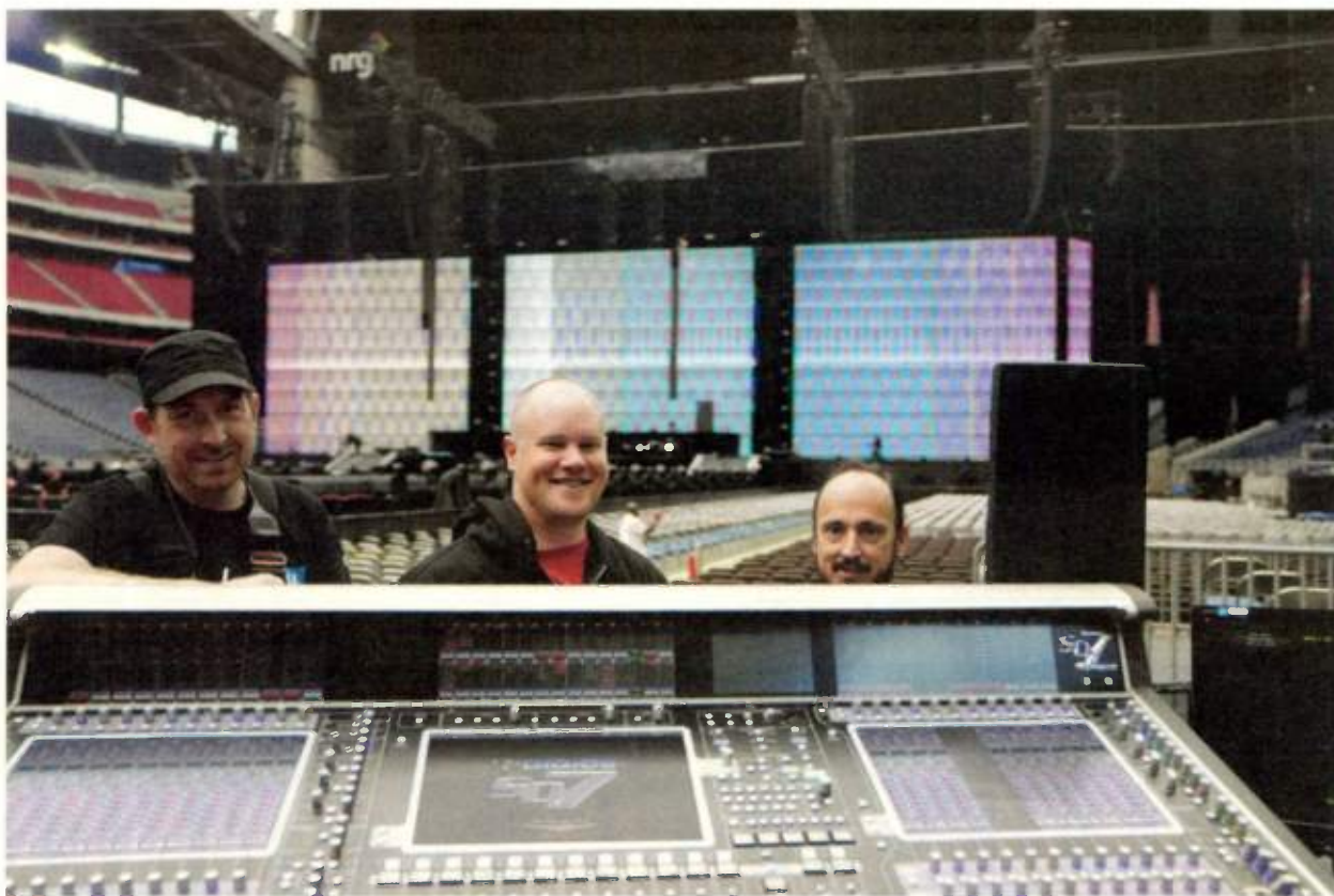
(L-R) James Berry and monitor tech Chris Bellamy at the tour's two DiGiCo SD7 monitor desks for the artists, with Jimmy Corbin in the background at his two band SD7s
