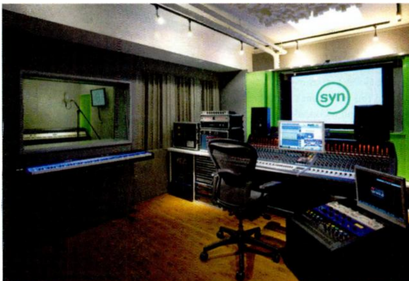
SYN's Tokyo studio sports Amphion monitors and a 32-channel AMS Neve Genesys console with Pro Tools HDX.
