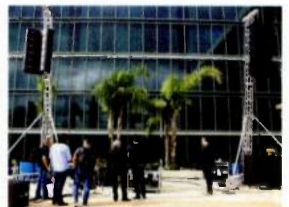
EAW Anna (left) and Bose Professional ShowMatch line array systems were hung from 25-foot ground-support towers temporarily installed on the roof of the Anaheim Hilton Hotel for the Line Array Loudspeaker System Academy.
