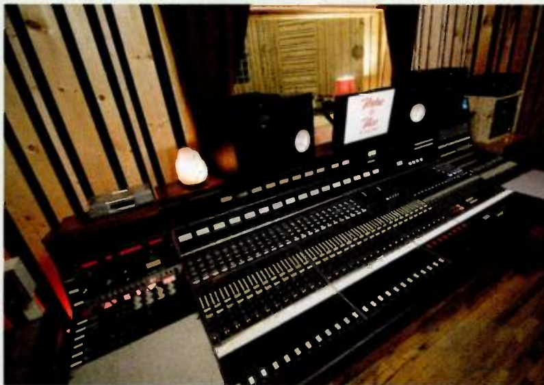
The 8-bus console, featuring 24 channels of 1084 modules with a pair of 2254 compressors, was installed in late 2017.
