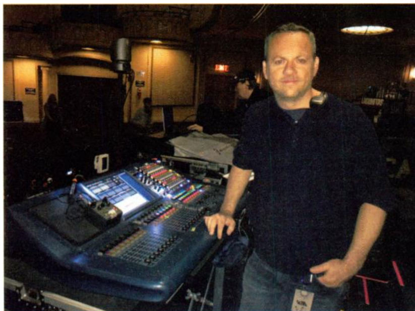
Michael Versteegt mixes SOJA on the band's Midas Pro2 console, using a Strymon El Capistan dTape Echo guitar pedal (at left) for dub effects.
