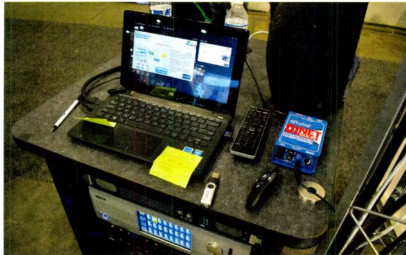
Ensuring that every device a presenter brought along could be integrated into a presentation, the IP Theater made use of a Radial DiNet DAN-TX Dante Network DI at stageside.
