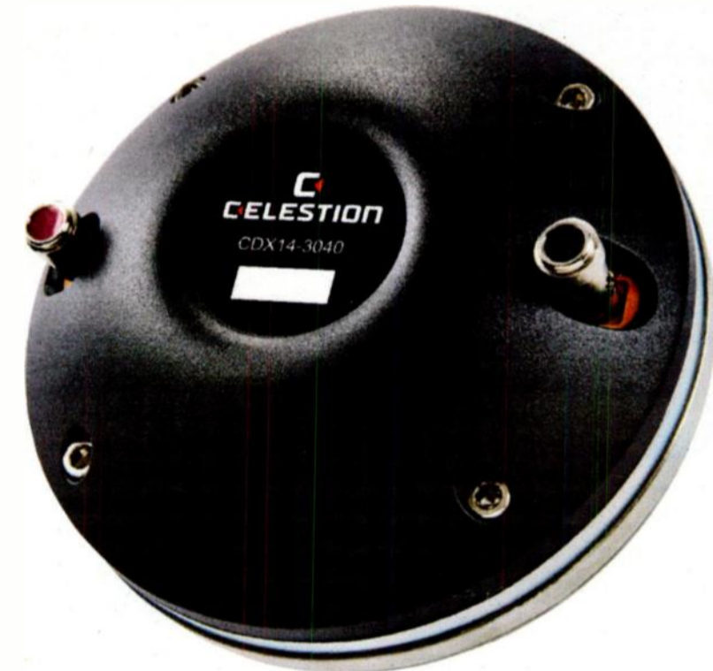
The neodymium-based CDX14-3040 has a 1.4-inch exit, a single-piece titanium diaphragm, 3-inch edge-wound copper-clad aluminum voice coil, and an annular three-slot phase plug.
