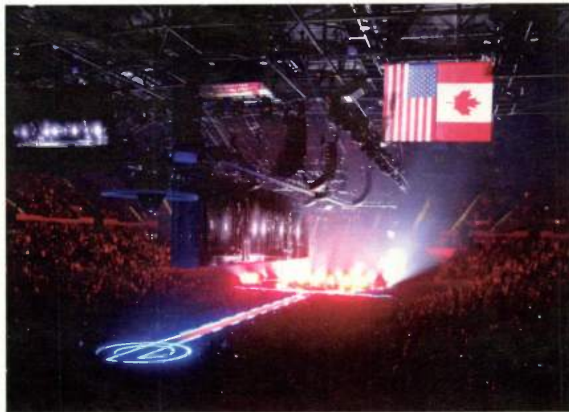
An omnipresent stereo image is achieved throughout the venue by a dozen Clair Cohesion CO-12 hangs that provide alternate left-right feeds around the perimeter of the arena.
