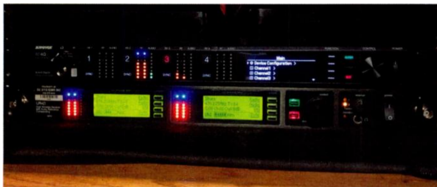
Placement atop an older Shure UR4D receiver during a production of Les Misérables inadvertently highlighted the extensive metering of the Axient Digital AD4Q.
