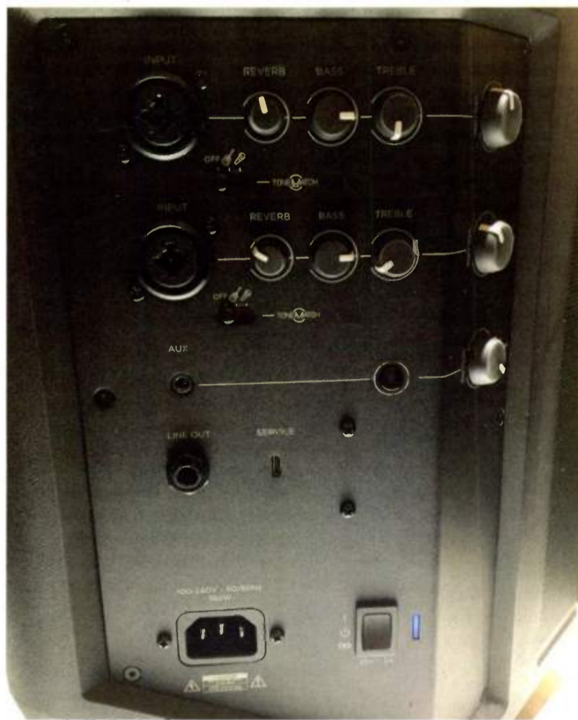
A three-channel mixer offers ToneMatch and Bluetooth connectivity, as well as Auto EQ that varies depending on the physical positioning of the enclosure.
