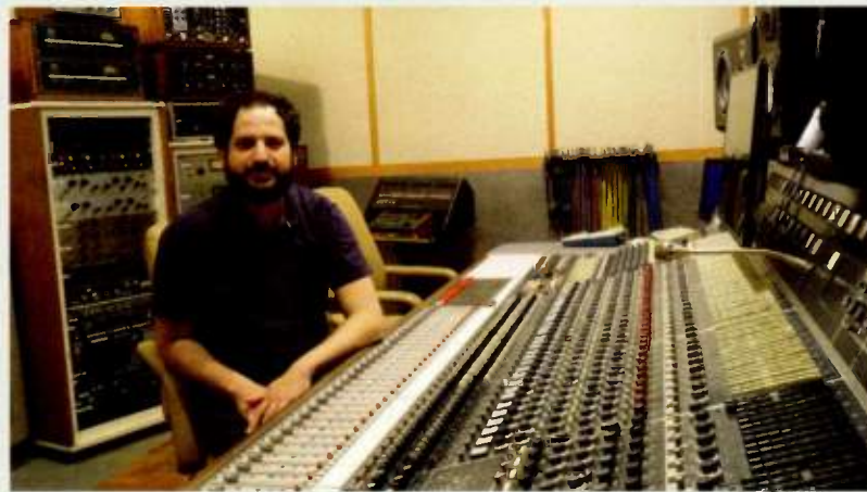
Independent engineer Will Chason at the classic 38-input Neve 8038 with Flying Faders automation installed in Hyde Street’s flagship Studio A
