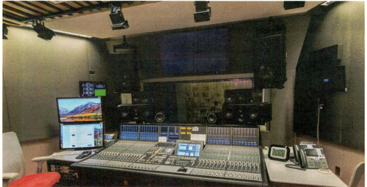
Every flavor of I/O is available in the performance studio, with recording over MADI to a 64-channel Avid Pro Tools system.
