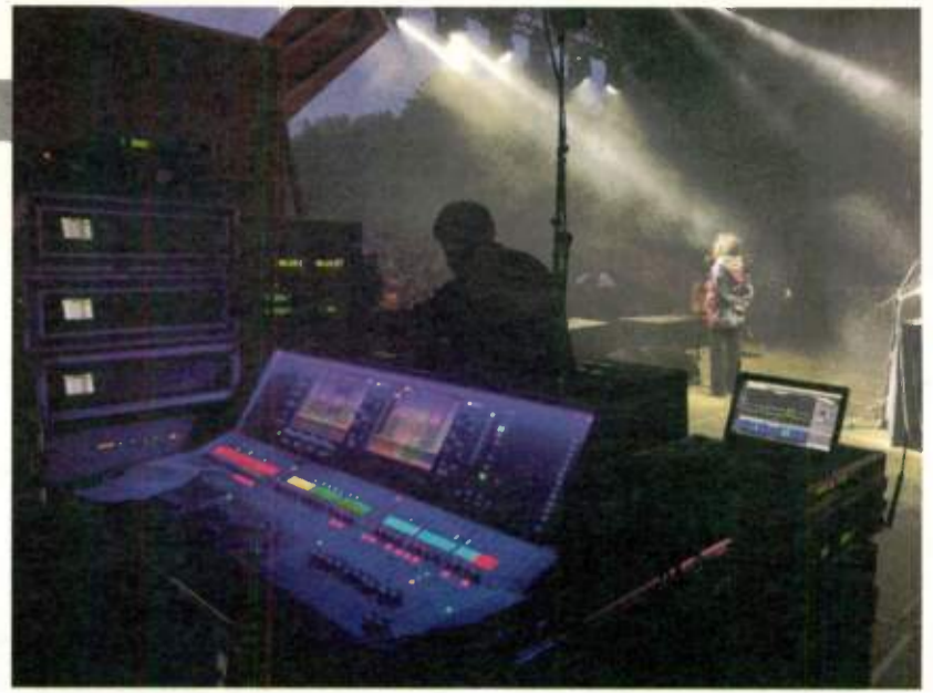
The main stage featured two dLive S7000s, one of which is pictured, and two DM64 MixRacks paired with three Dante cards.
