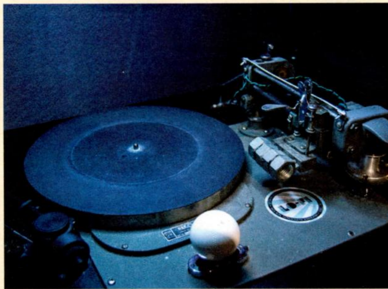
Leesta Vall Sound Recordings has cut more than 700 sessions live to vinyl using an ancient Presto K8 portable vinyl record lathe.
