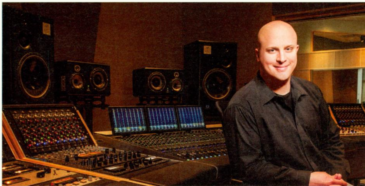
Mark Hornsby, vice president of operations and senior producer/engineer, sits at Sweetwater Studios' "Neve 6," a mash-up of an Avid S6 control surface flanked by Rupert Neve Designs 5088 desk Shelford input modules.
