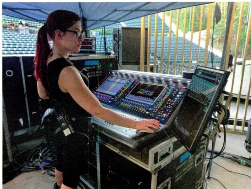
Loreen Bohannon mixes monitors for Lizzo on Clair Global's DiGiCo SD12 96 desk.
