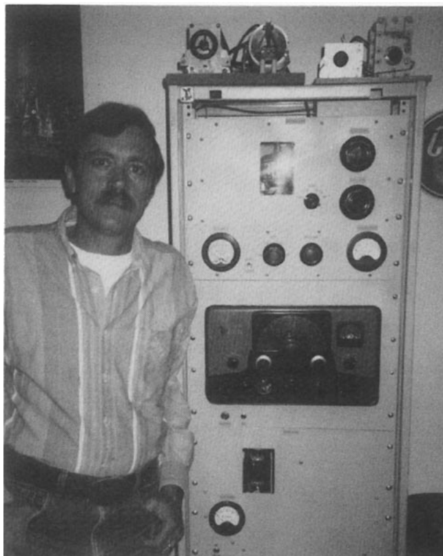
Bill and his mighty homebrew 1 KW plate modulated AM ham radio transmitter—304TL triode modulated by push-pull 810s. The modulator deck is good for 700W of audio at 5% THD!
