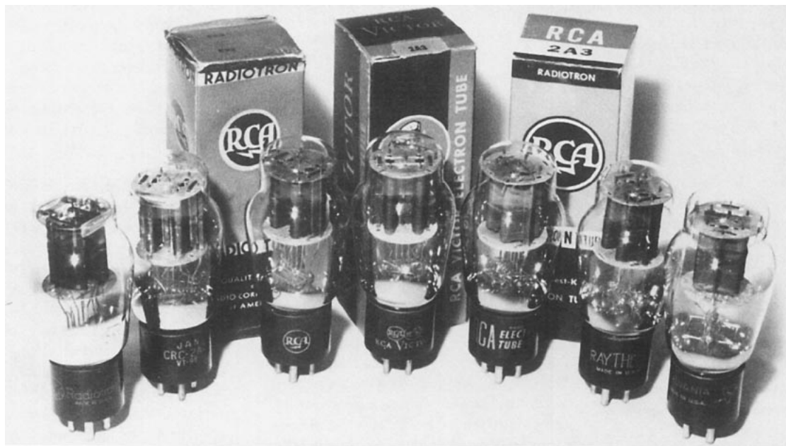
RCA 2A3 tubes in chronological order: Red-label from May-June 1937, followed (left to right) by wartime, late 1940s, and 1950s production.
