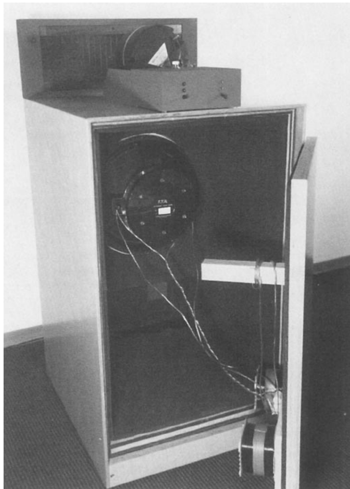
Highpass filter with 0.2 dB per step attenuator, 1.2 mH/0.13 Ohm DCR coil, and five PP caps bypassed with a tinfoil cap shown mounted behind the TAD horn
