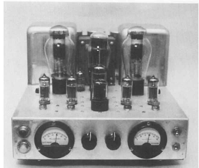
Raul Gil's latest project. . . Direct coupled SE 300B with 5692 + 6SL7 drivers regulated by four 6S4s. The 300Bs are regulated by a 6AS7.
