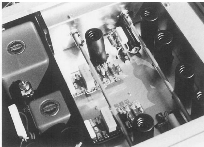
Interior view of PA-7000 preamplifier showing compartmentalized subchassis construction technique for superior noise elimination
