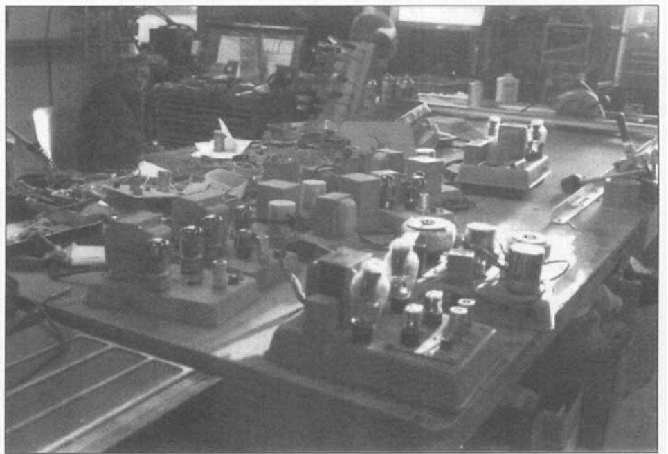
The workshop : One 300B amp and power supply in foreground featuring Al’s trademark cake pan chassis style. Wood shop in the back.
