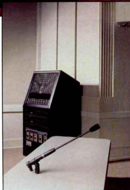
The professor's console. Note control panel in shape of classroom.
