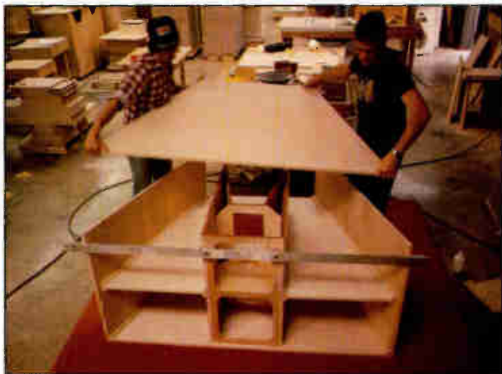
Under construction, this shows the seven-foot-long folded horn design from Klipsch.
