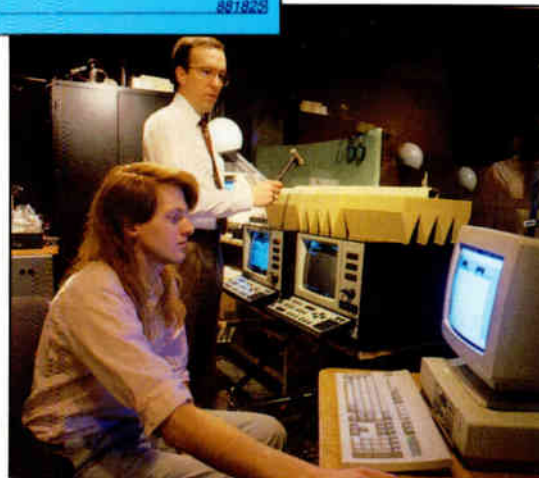
Modal Testing with Impact Hammer.
