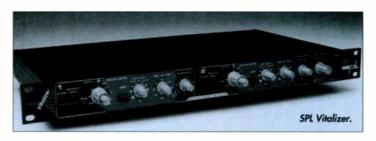
top end was relatively dull, and vocal diction suffered slightly. Using the Vitalizer to accentuate the high mids at around 2.5kHz, and the harmonics control to restore missing sibilants, lyrics regained clarity, and backing vocals which were hitherto almost lost became quite audible. This process
