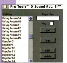
GRM Tools Settings Control Window: The control settings can be saved here for each algorithm. A useful selection of factory settings, which you can load into this window, is provided on disk.
