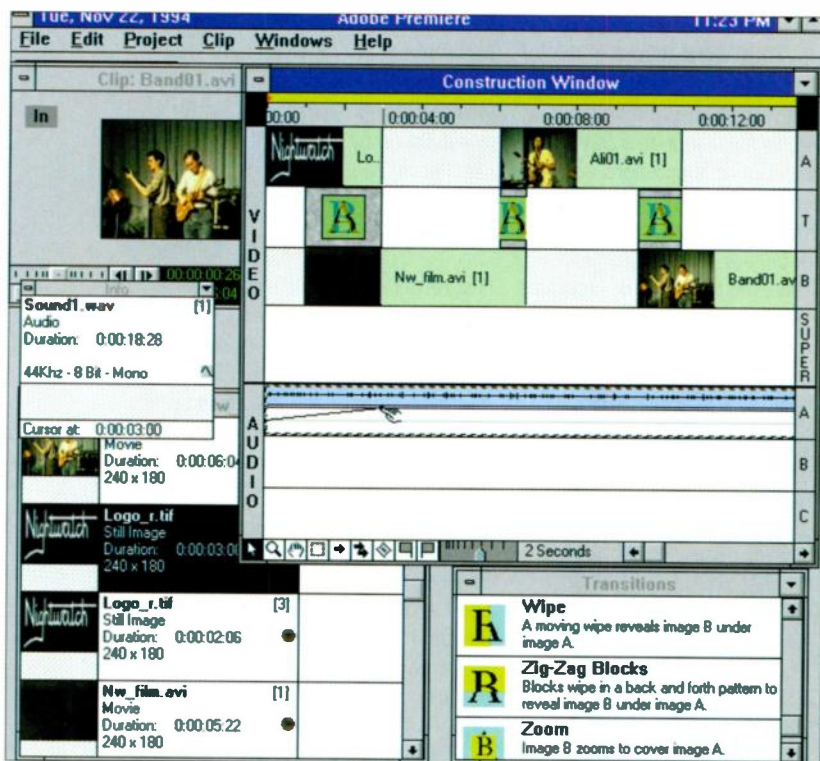
The Adobe Premiere software provides some advanced editing facilities. The pointing 'hand' cursor shows an audio fade being adjusted graphically.
