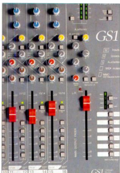
Allen & Heath GS1 Mixer p78 Allen & Heath's latest model offers MIDI Machine Control and onboard muting in a usefully compact package.
