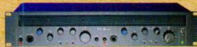
Dual Pentode Valve Pre-amp Transformer coupled mic input, +48v phantom power, input/output gain controls, front panel instrument input, Phase reverse switch, Filters.
